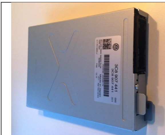
Figure 7 J722 control unit.
