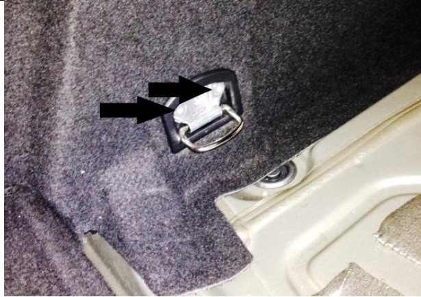
Figure 15 Hidden screws in the lashing eye to untighten when removing the right side trim of the luggage compartment.
