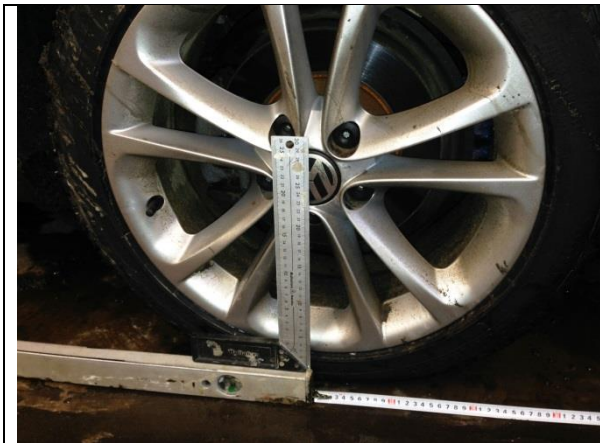
Figure 41 Measuring distance from rear axle (centre) to calibration board (not shown in this picture).
