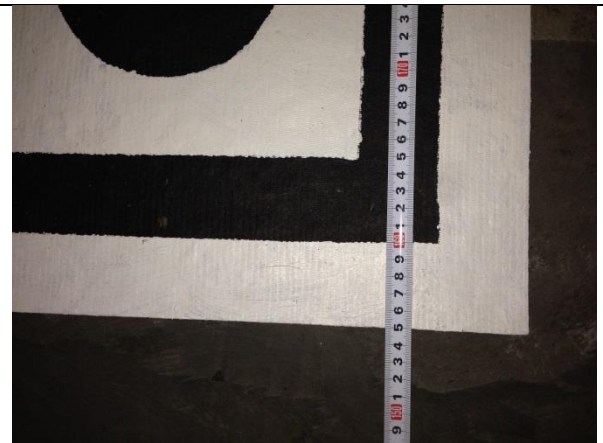
Figure 42 Measure distance from the rear axle to the black border (closest to the car). Here distance is 1600 mm.
