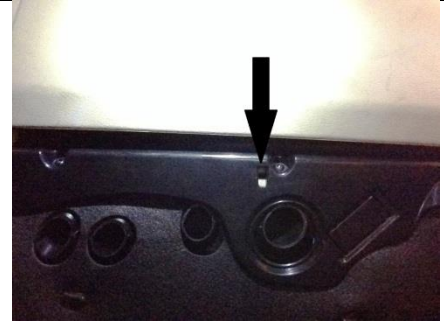
Figure 31 Glove compartment release hatch.
