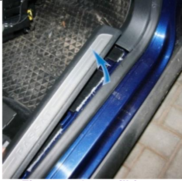
Figure 29 Open sill front.
