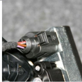
Figure 23 The art no. 37112 cable connects to the four pin connector on the VW emblem/camera unit.
