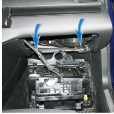
Figure 30 Remove glove compartment by unscrewing screws and releasing hatch.
