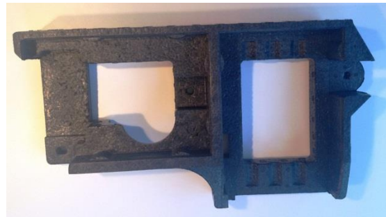
Figure 8 Control unit retainer (you already have this if you have a shock absorber regulator J250 controller – which most Passat CC probably have).
