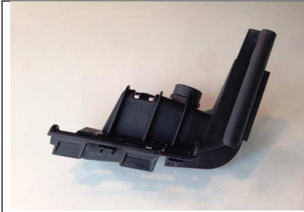
Figure 18 Rear lid strut cable guide VAG 3C8971616A.
