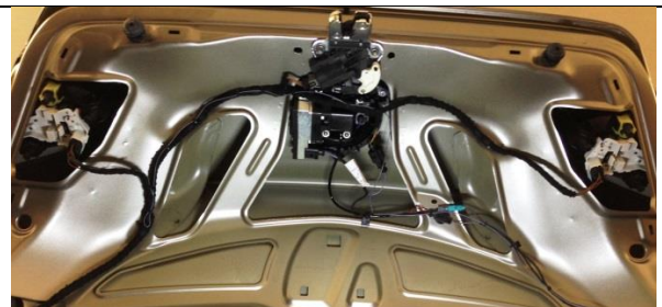
Figure 11 VW emblem/camera unit mounted, new cables routed.
