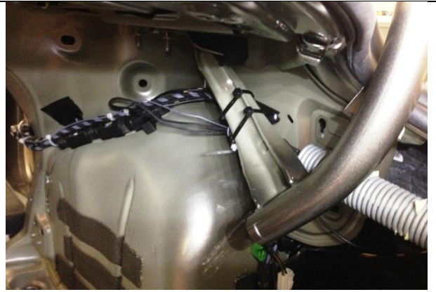
Figure 19 Rear lid strut cable guide (3D printed/homemade).
