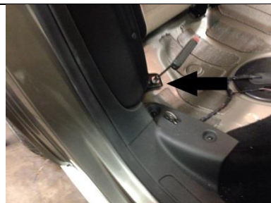
Figure 27 Rear seat padding removal bolt.
