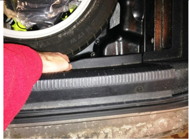
Figure 16 Remove the lock carrier trim by just lifting it straight up.
