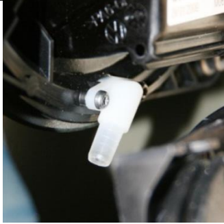
Figure 12 Swivel emblem drain pipe nipple.
