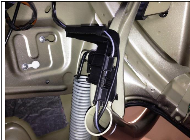
Figure 20 Cables routed through rear lid strut and through the VAG 3C8-971-616-A cable guide (picture taken from inside luggage compartment looking up).
