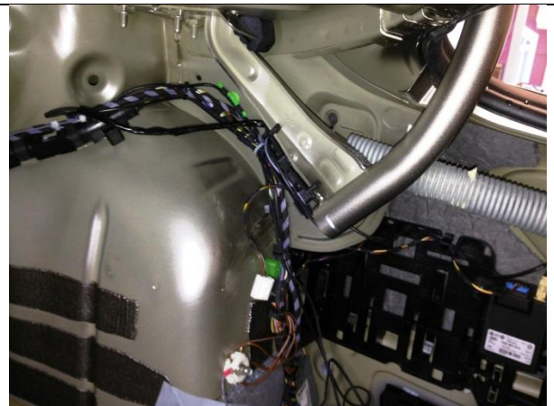
Figure 21 Pushi cables through the rear lid right strut.
