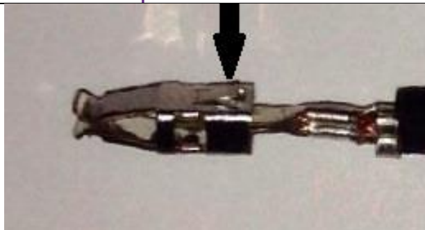
Figure 37 Notice the flukes that have to be depressed by a pin removal tool.
